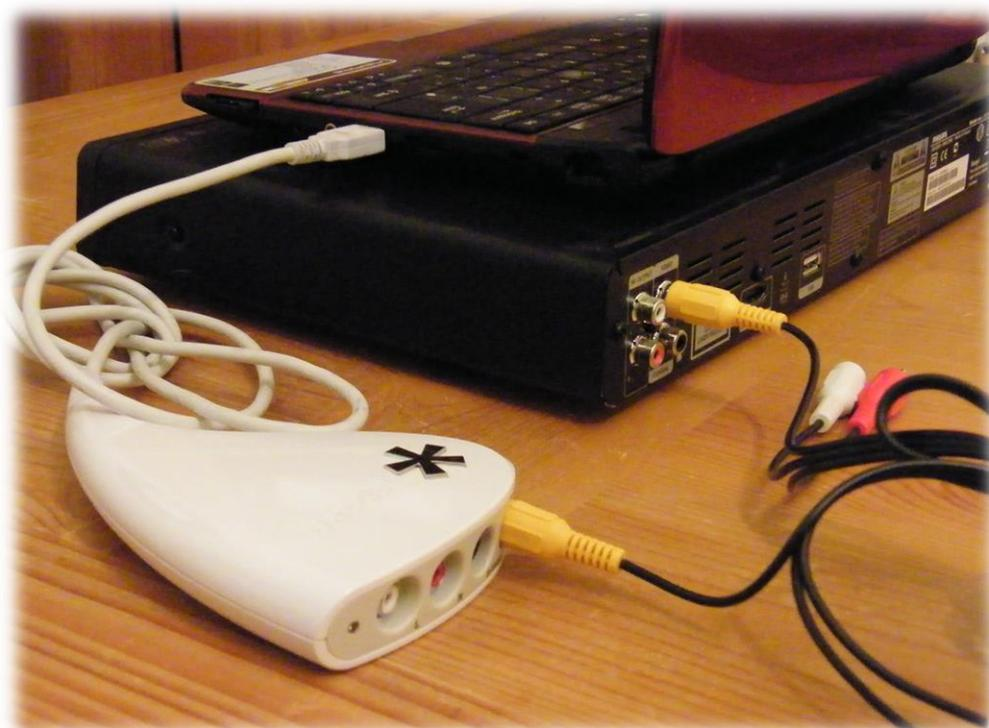
In Fig 1 the Composite output is from a DVD player but the principle is the same as it would be if you were using the composite output from your camera control unit. We have used a Pinnacle Dazzle DVC100 composite to USB converter to connect to the laptop.
